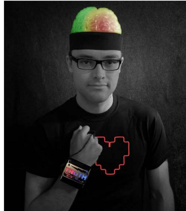
**figure 1.** Clothing with embedded circuitry to measure and display biological signals of the wearer. The Truth Wristband displays the wearer's emotional responses by measuring the galvanic skin response. The Heart-felt Shirt flashes with the wearer's heart beat. The Thinking Cap displays changes in neuronal synchrony on 6 modular RGB arrays.
