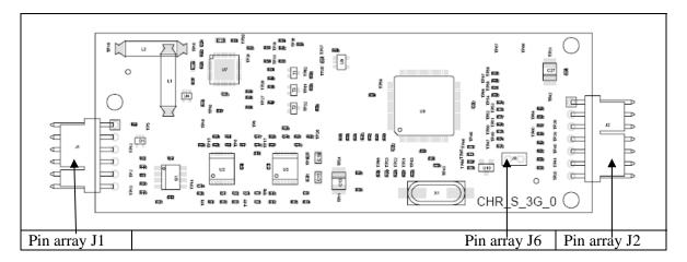
Detailed pin description can be found below. Square on each pin array defines the pin number 1.
